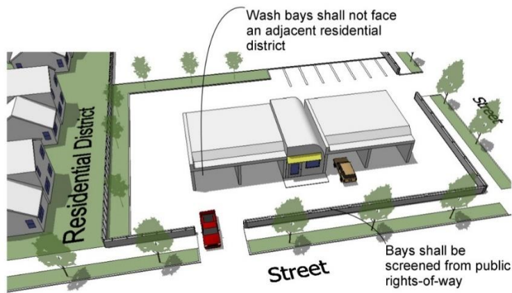
Figure 36: Car Wash Bay Location; 17.7.6.3:A
