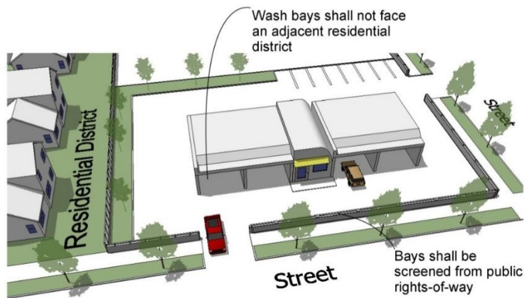
Figure 36: Car Wash Bay Location; 17.7.6.3:A
