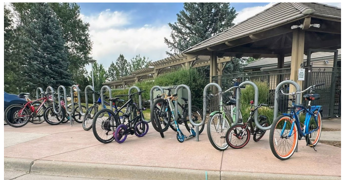
Figure D-3: Wave racks can provide high-volume bike parking with minimal drilling required, but offer less security than other racks.
