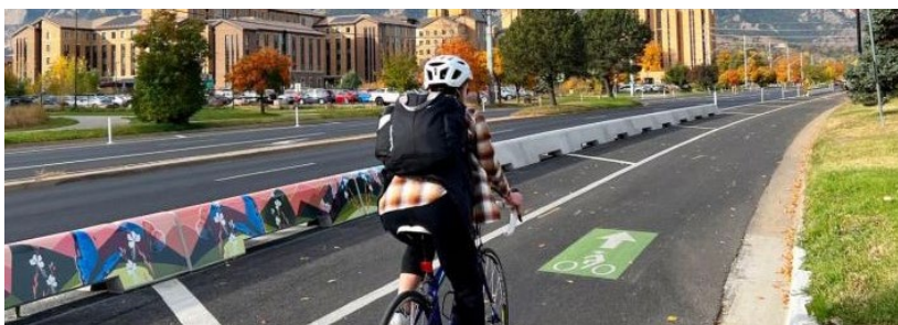
Figure E-7: A concrete barrier protected bike lane with a painted mural on Baseline Rd in Boulder, 2023.
