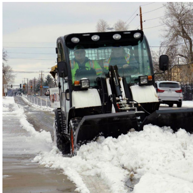
Figure 21: Scaled-down plowing equipment clears a separated bike lane.
