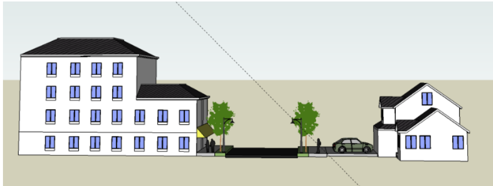
Figure 17.5.7: Bulk Plane Height Transition
