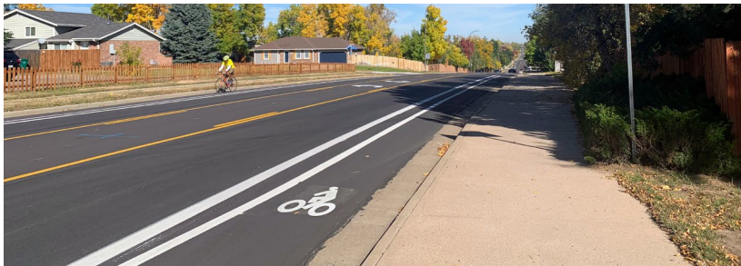
Figure E-3: A buffered bike lane on Garrison St near Green Gables Park in 2023 before it was upgraded to a separated bike lane.
