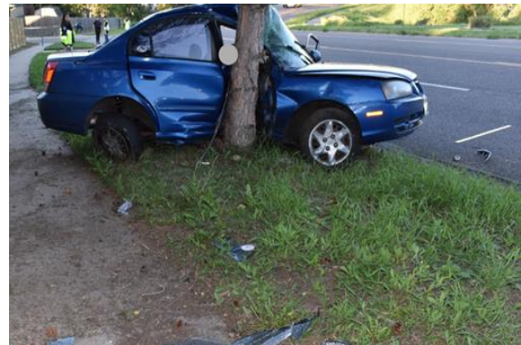
Exhibit 7 - Trees with a diameter as small as 4 inches can be fatal in a vehicle collision. Maintaining a clear zone behind the curb is essential to provide room for correction if a motorist loses control, helping to prevent such incidents from resulting in loss of life.
